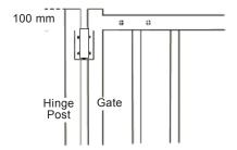
Step 3 - Fix the gate to the hinge post. Support the gate on blocks so that the gate is level with the top of the hinge post. Check the gap under the gate is not greater than 100mm. Now tek screw the hinges to the hinge post. The hinge will automatically set the gap to 20mm provided it is pushed firmly against the hinge post when tek screwing.
